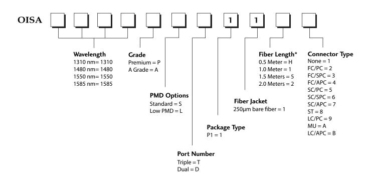
\* The tolerance of fiber length is +/-0.1m. 1 meter is standard. The lead-time for special fiber length will be longer.
